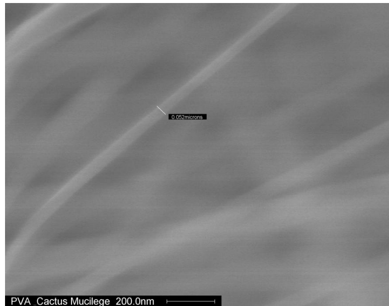
Figure 19: SEM Image at 70Kx of 11% PVA and Mucilage (70:30) PVA:Mucilage Fiber Measured at 52nm.
